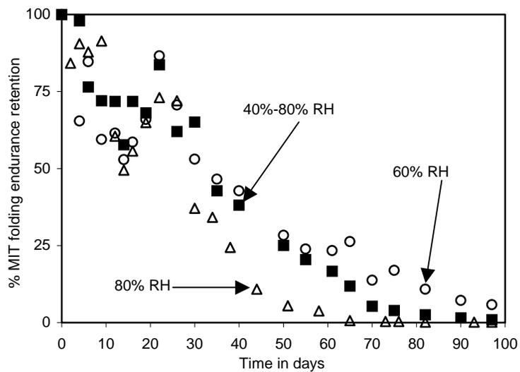
Figure 9. Effect of cycling RH at 70°C on MIT folding endurance of Paper 7. Percent retention versus incubation time.
