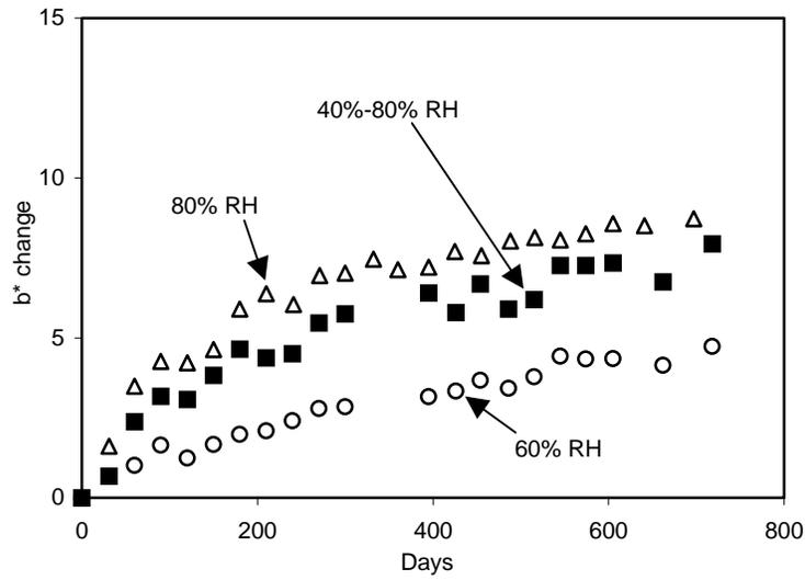
Figure 11. Effect of cycling RH at 50°C on Paper 8 discoloration.  $b^*$  change versus incubation time. Initial  $b^*$  value: 11.2.
