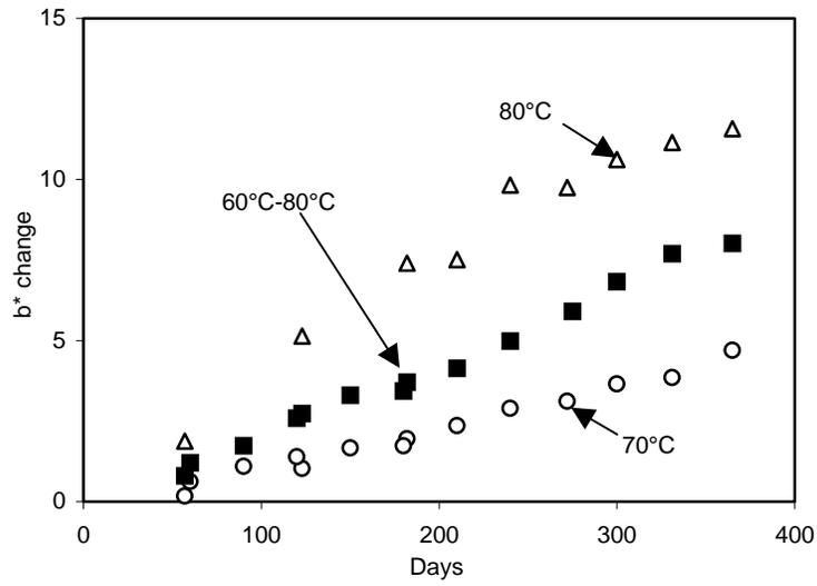
Figure 15. Effect of cycling temperature on Paper 5 discoloration at 50% RH. b\* change versus incubation time. Initial b\* value: -1.
