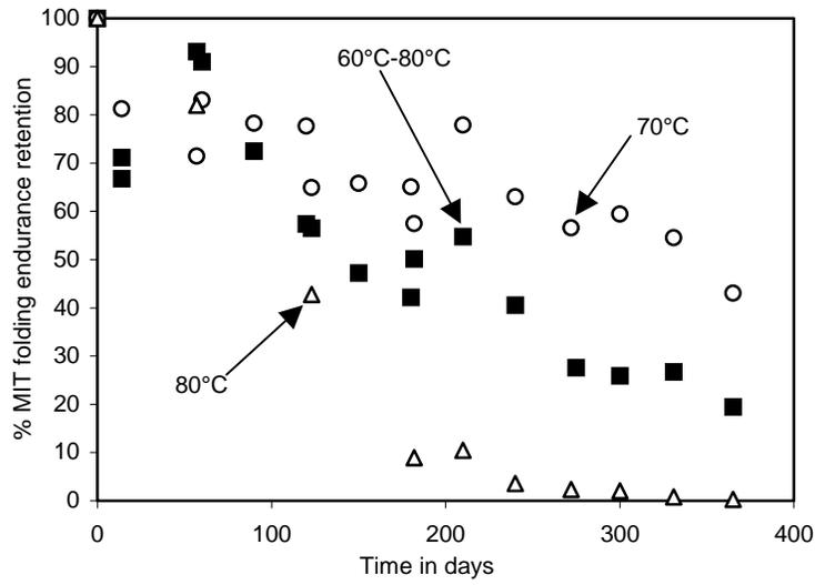
Figure 18. Effect of cycling temperature at 50% RH on MIT folding endurance of Paper 5. Percent retention versus incubation time.
