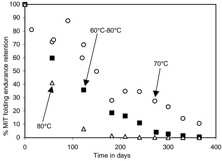
Figure 20. Effect of cycling temperature at 50% RH on MIT folding endurance of Paper 8. Percent retention versus incubation time.
