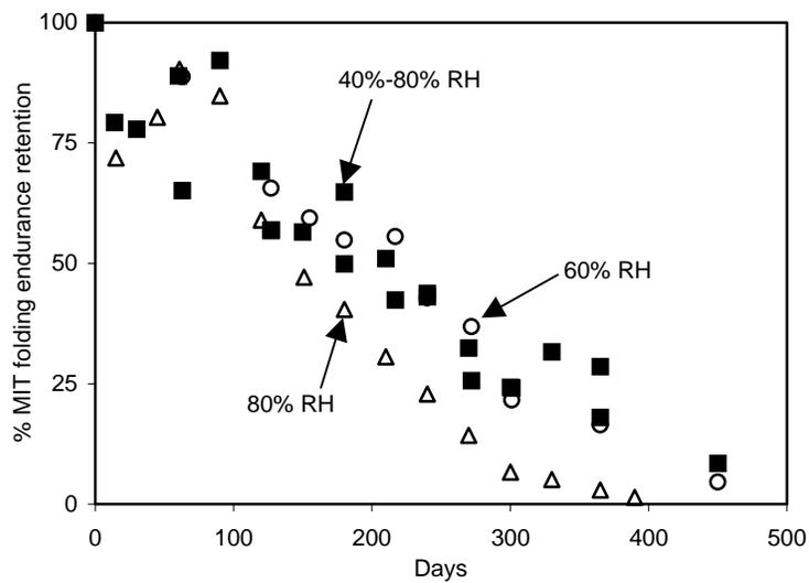
Figure 13. Effect of cycling RH at 70°C on MIT folding endurance retention of Paper 8. Percent retention versus incubation time.
