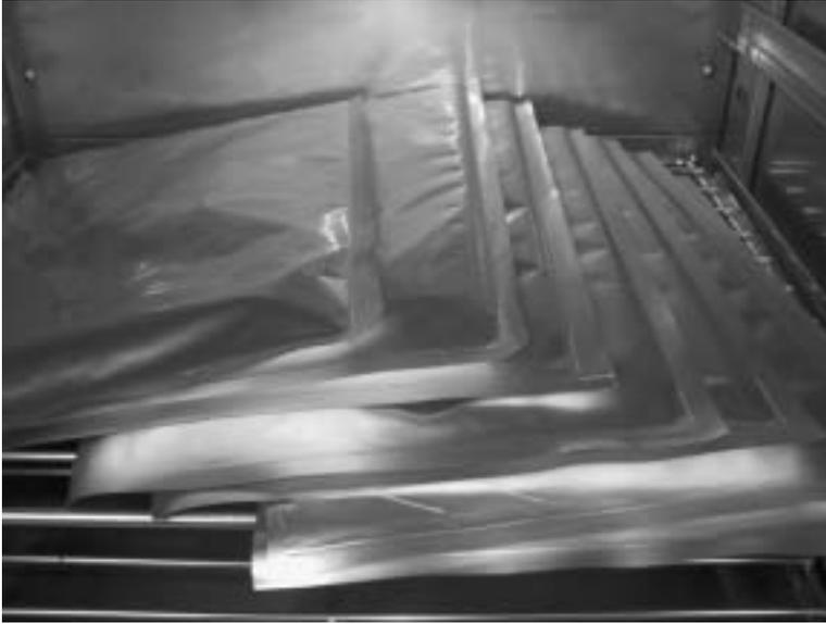
*Figure 4. After moisture conditioning, 100-sheet stacks of paper were heat-sealed inside two aluminum foil bags and incubated under three different temperature conditions to study the effect of cycling temperature at constant moisture content.*
