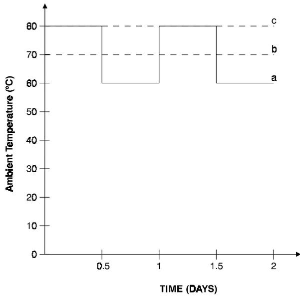
Figure 14. Temperature conditions. (a) Cycling between 60°C and 80°C. (b) Static at 70°C. (c) Static at 80°C.
