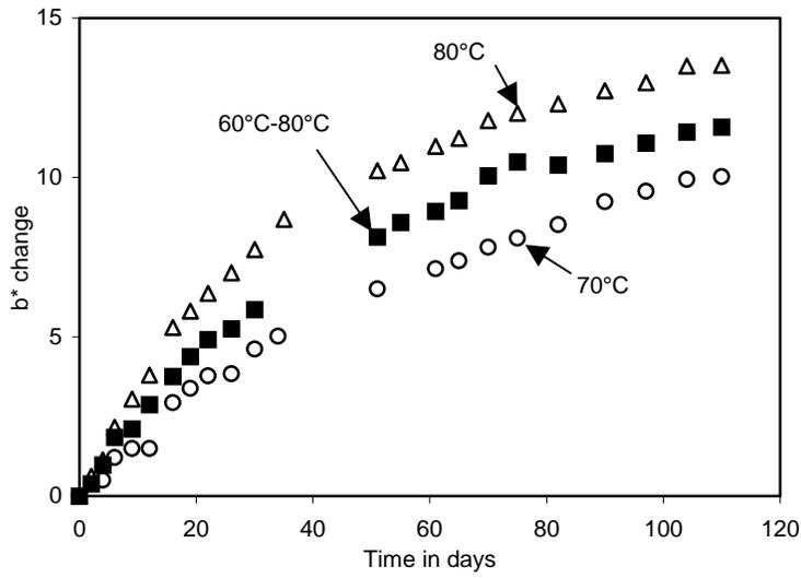
Figure 16. Effect of cycling temperature at 50% RH on Paper 7 discoloration.  $b^*$  change versus incubation time. Initial  $b^*$  value: 12.1.
