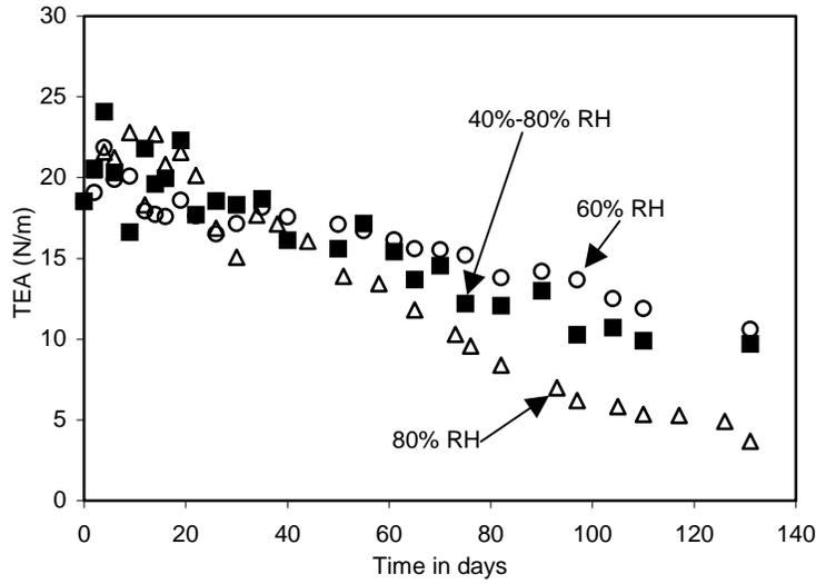
Figure 10. Effect of cycling RH at 70°C on tensile absorption energy (TEA) of Paper 7.
