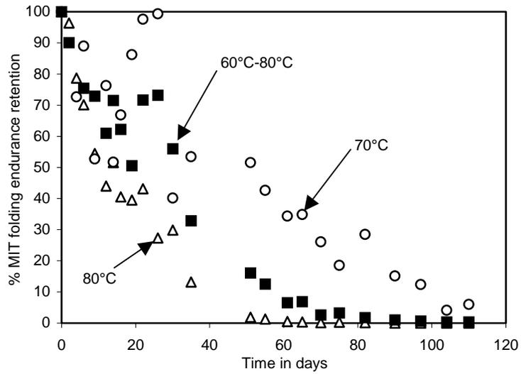
Figure 19. Effect of cycling temperature at 50% RH on MIT folding endurance of Paper 7. Percent retention versus incubation time.
