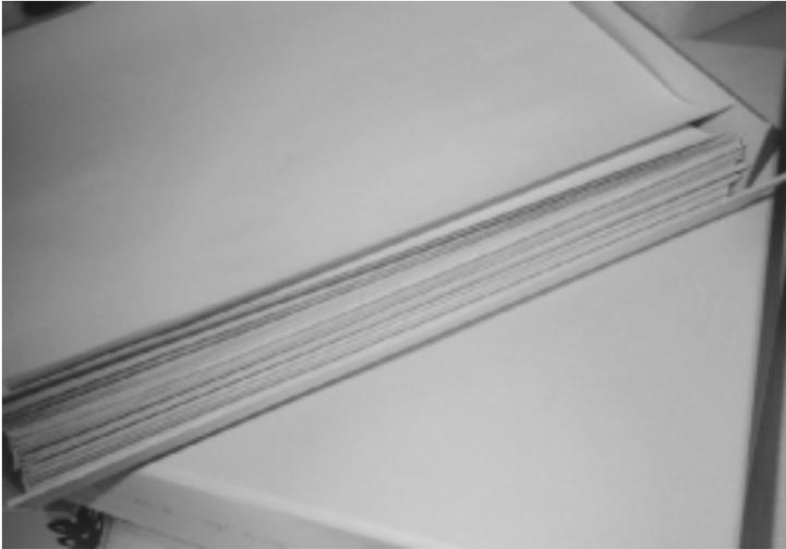
*Figure 2. One-hundred-sheet stacks of paper were enclosed in drop-front cardboard boxes to study the effect of cycling RH at constant temperature and cycling temperature at constant RH. Measurements were made on sheets pulled from the middle of each stack.*
