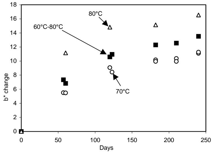
Figure 22. Effect of cycling temperature at constant moisture content on Paper 8 discoloration. Paper initially conditioned to 21°C, 50% RH.  $b^*$  change versus incubation time. Initial  $b^*$  value: 11.2.
