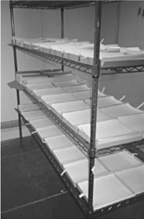
*Figure 1. Paper stacks were moisture-conditioned at 21°C, 50% RH prior to incubation under various conditions.*
