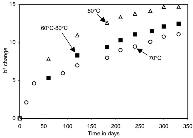
Figure 17. Effect of cycling temperature at 50% RH on Paper 8 discoloration.  $b^*$  change versus incubation time. Initial  $b^*$  value: 11.2.
