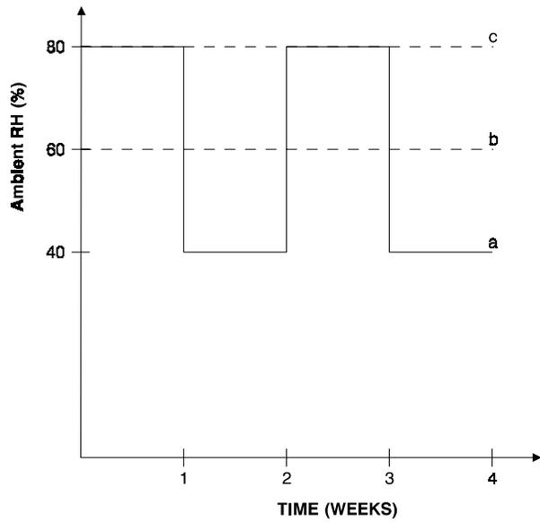
Figure 5: Humidity cycling conditions. (a) Cycling between 40% and 80% RH. (b) Static at 60% RH. (c) Static at 80% RH.
