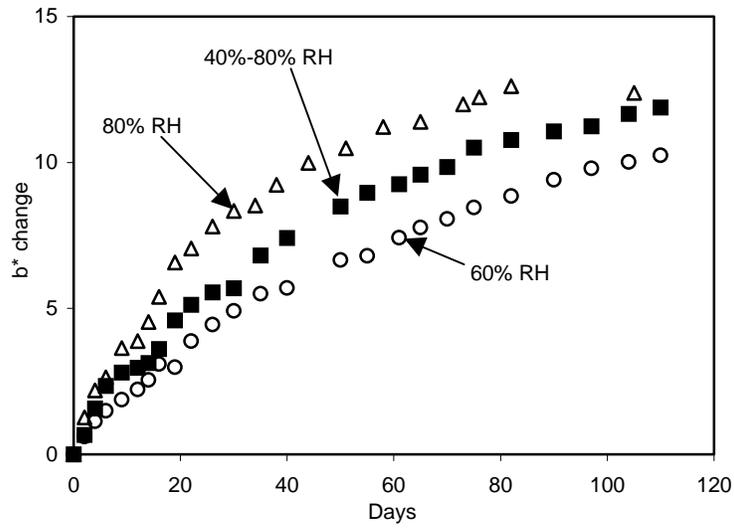
Figure 7. Effect of cycling RH at 70°C on Paper 7 discoloration. b\* change versus incubation time. Initial b\* value: 12.1.
