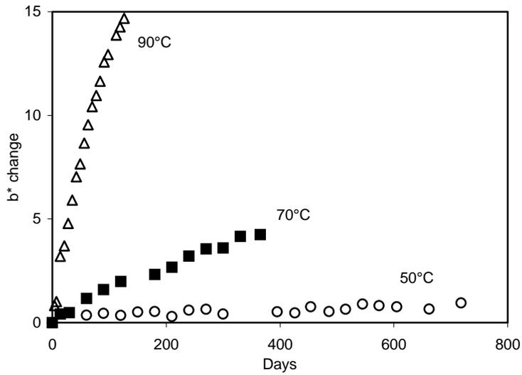
Figure 6: Effect of temperature on Paper 5 discoloration at 50°C, 70°C, and 90°C under cycling humidity conditions between 40% RH and 80% RH (two-week cycle).  $b^*$  change versus incubation time. Initial  $b^*$  value: -1.
