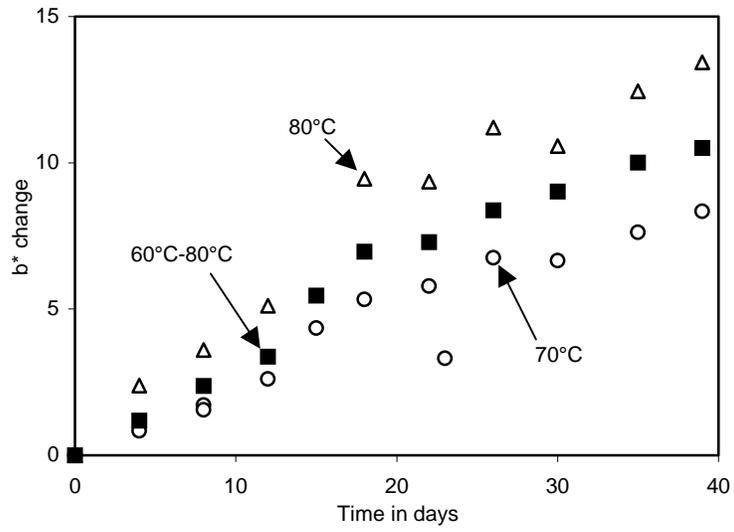
Figure 21. Effect of cycling temperature at constant moisture content on Paper 7 discoloration. Paper initially conditioned to 21°C, 50% RH.  $b^*$  change versus incubation time. Initial  $b^*$  value: 12.1.
