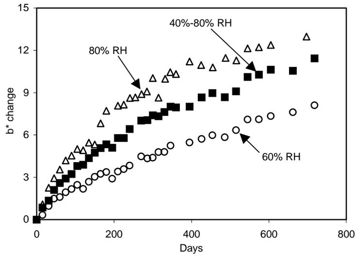
Figure 8. Effect of cycling RH at 50°C on Paper 7 discoloration. b\* change versus incubation time. Initial b\* value: 12.1.
