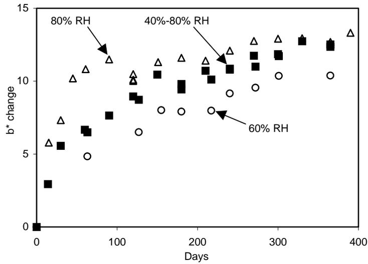
Figure 12. Effect of cycling RH at 70°C on Paper 8 discoloration.  $b^*$  change versus incubation time. Initial  $b^*$  value: 11.2.
