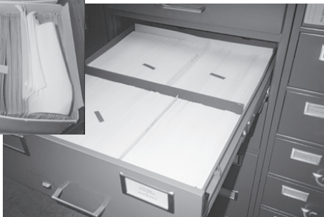
Figure 3. For film stored in a metal cabinet, strips are placed on top of film stacks and drawer is closed for the required exposure period.
